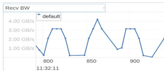
NVLink utilization GPU0 to GPU1
