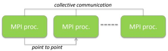
An MPI program is a set of autonomous processes that exchange data through message passing
