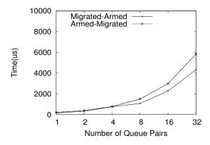
Figure 5. Timings for different transition states in APM, Small Number of QPs
