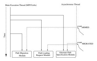
Figure 4. Interaction of Network Fault Tolerance Modules with Main Execution Thread and Asynchronous Thread
