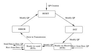
Figure 1. QP Communication State Diagram
