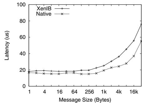
Figure 14: Send/Receive Latency Using Blocking VERBS Functions
