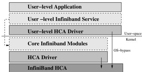
Figure 3: Architectural overview of OpenIB Gen2 stack
