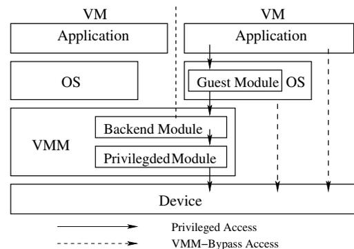
Figure 4: VM-Bypass I/O (I/O Handled by VMM Directly)
