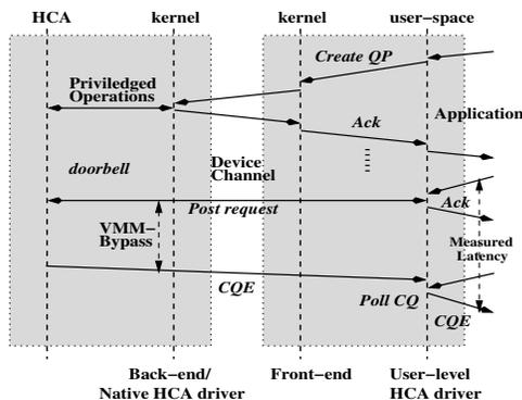
Figure 8: Working flow of the VMM-bypass Xen-IB driver
