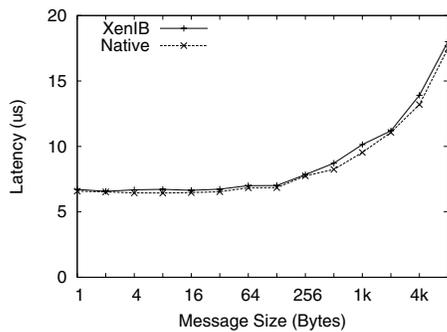
Figure 10: InfiniBand Send/Receive Latency
