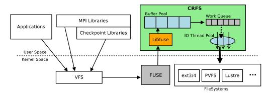
Fig. 4. CRFS Design Diagram
