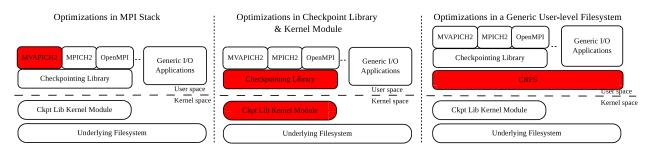
Fig. 1. Checkpoint/Restart Optimizations at Different Levels. Optimizations are Performed in Highlighted Components. Optimizations in MPI stack can only benefit certain MPI implementation. Optimizations in checkpoint library and Kernel module are not portable. Optimizations in a generic user-level filesystem is portable and can transparently benefit a wide range of MPI stacks and applications.
