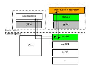
Fig. 2. FUSE Architecture (Courtesy of [15])
