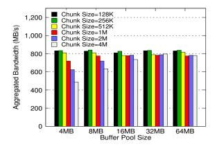
Fig. 5. CRFS Raw Write Bandwidth (8 processes on a single node)
