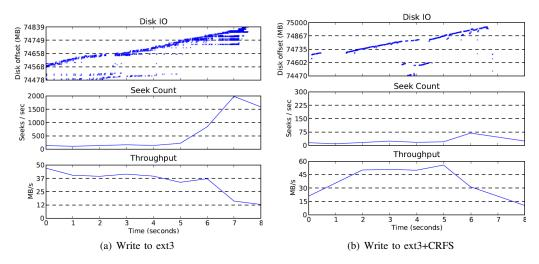
Fig. 10. Block IO Layer Trace on One Node. Checkpoint Writing of LU.C.64 on 8 Nodes, ext3
