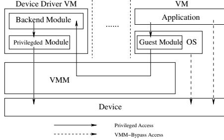
**Figure 4: VMM-Bypass I/O**
