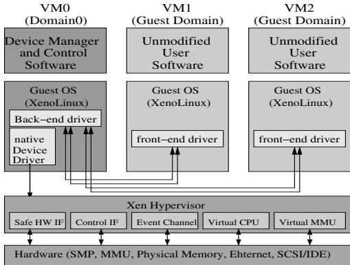
**Figure 1:** The structure of the Xen hypervisor, hosting three xenoLinux operating systems
