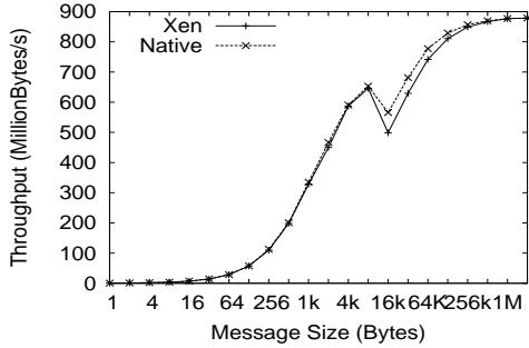
**Figure 11: MPI bandwidth test without registration cache**
