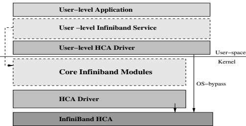
**Figure 2:** Architectural overview of OpenIB Gen2 stack
