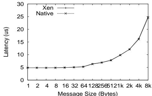
Figure 7: MPI latency test
