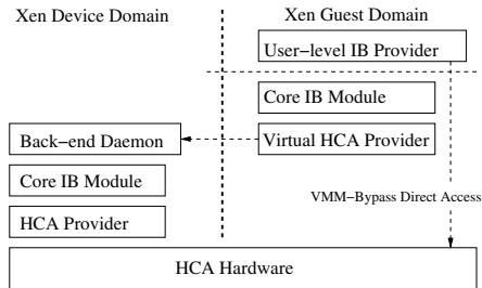
**Figure 6: Xen-IB Architecture: Virtualizing InfiniBand with VMM-bypass I/O**
