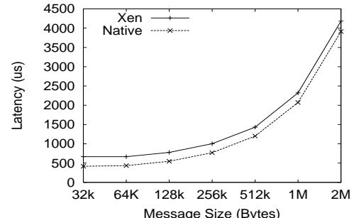
Figure 10: MPI latency test without registration cache (large messages)
