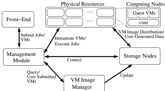
**Figure 5: Framework for Cluster with Virtual Machine Environment**
