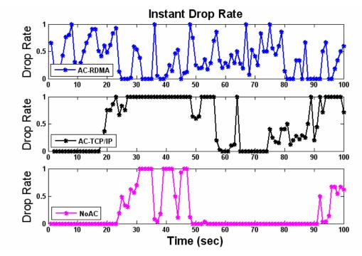
AC-RDMA gets the load information timely, while AC-TCP/IP sometimes reads the stale information due to the slow response from overloaded servers in TCP/IP communication
