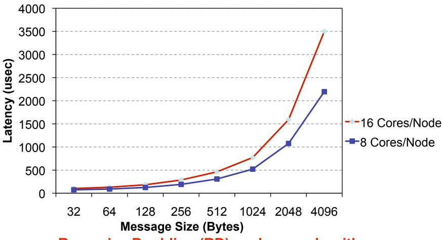
Recursive Doubling (RD) scales poorly with increasing core counts
