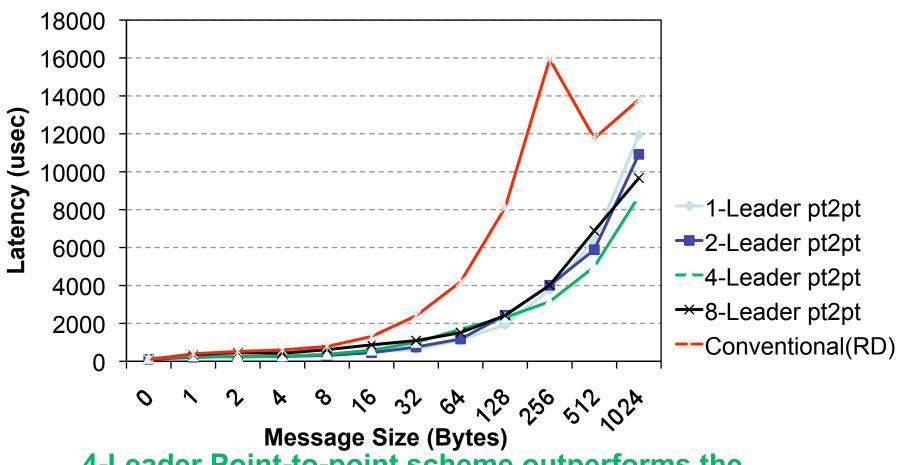
4-Leader Point-to-point scheme outperforms the recursive doubling method on 1024 processes on the TACC Ranger
