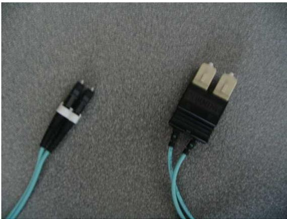
Figure 1.12: InfiniBand Fibre Cables
