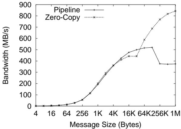
**Figure 11. MPI Bandwidth with Zero-Copy and Pipelining**
