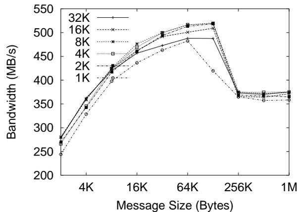
**Figure 9. MPI Bandwidth with Pipelining (Different Chunk Sizes)**
