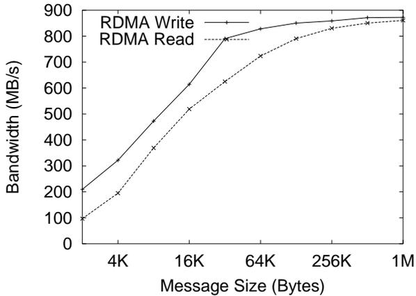
Figure 15. InfiniBand Bandwidth
