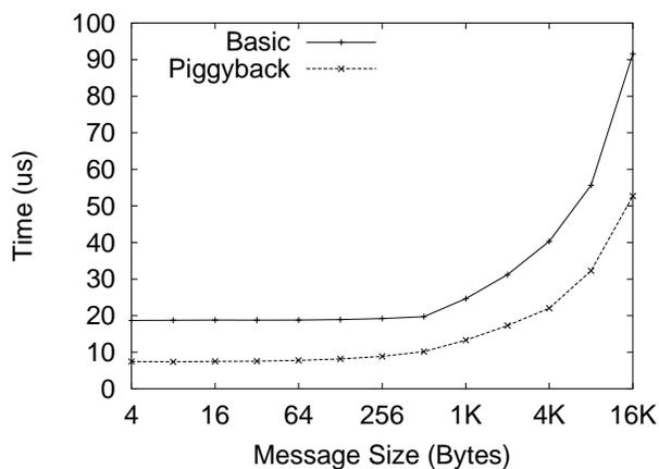
**Figure 6. MPI Small Message Latency with Piggybacking**
