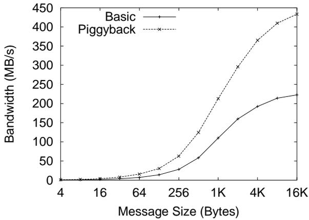
**Figure 7. MPI Small Message Bandwidth with Piggybacking**
